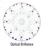
Optical Symmetry Analysis: The colored areas of the symmetry image are indications of light handling ability, giving a visual representation of proportions and facet alignment.
